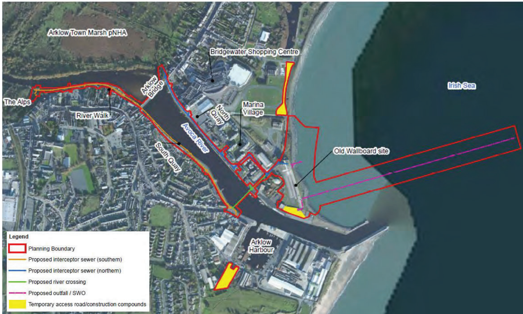
Figure 2.27 Overview of Main Elements of WwTP Project. Not to Scale. Extracted from WwTP EIAR
